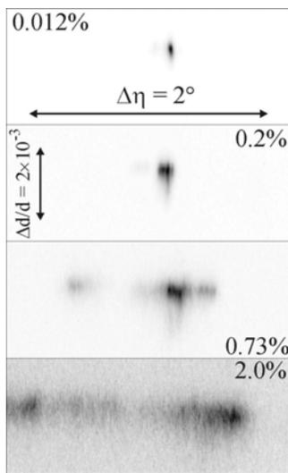
Fig. 2. Raw detector images of a selected diffraction spot. The tensile strains are indicated. The vertical axis—measuring the lattice strain—is enlarged by a factor of 5 against the horizontal direction, which is tangential to the diffraction ring. The diffraction spot to the left in the bottom image has rotated into the detector field during the last deformation step. The lattice strain and mosaicity scales are indicated.
