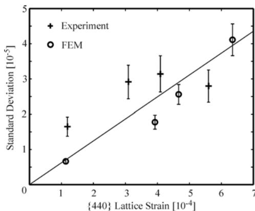
Fig. 3. Comparison of the experimental and FEM-simulated standard deviations of the {440} axial lattice strain components. The values are plotted versus the respective average axial lattice strains. A straight line obtained by linear regression is plotted as a guide to the eye.
