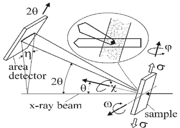
Fig. 1. Sketch of the experimental configuration with the stress-rig mounted on a Eulerian cradle. The orientation angles  $\varphi$ ,  $\chi$  and  $\omega$  are defined. The insert sketches the diffraction from an internal grain.  $\sigma$  indicates the direction of the applied tensile stress. Only the high resolution detector is show.
