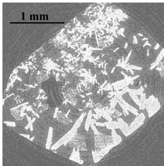
**Fig. 1.** Cross-section through a 3-D synchrotron X-ray  $\mu\text{-CT}$  volume of a young chimney collected from 9°N EPR. Sample was impregnated with epoxy; bright minerals are sulfides, darker minerals are sulfates; interstitial gray is pore space.
