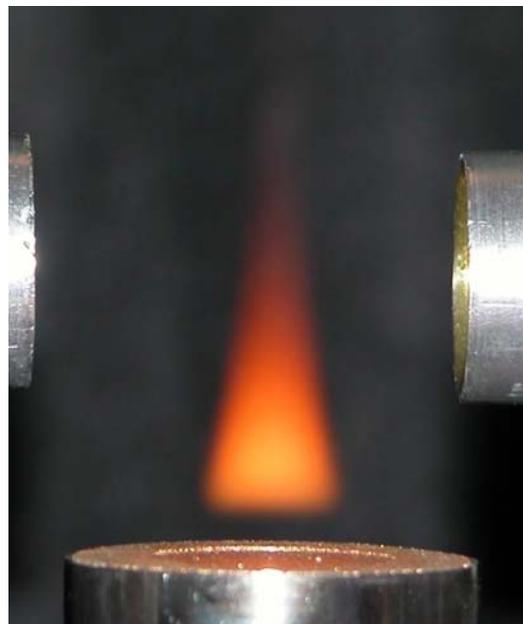
Fig. 1. Premixed flame of ethylene, oxygen, and argon. The x-ray beam is transported in vacuum by the two aluminum tubes.
