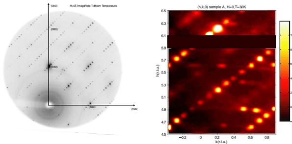
**Figure 3** High resolution image plate (left) and detector data (right) indicate the sample is not twinned. Based on the reciprocal space data, we choose a small range of  $(h, k, 0)$  zone under different fields and compare their differences.
