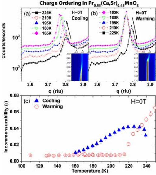
**Figure 2** Top panels: representative charge ordering peaks at different temperatures, the temperature evolution of peak position are plot in the insets. Bottom panel, incommensurability (defined as offset value from commensurate peak position) v.s. temperature as samle is thermal cycled. The high resolution X-ray experiments ensure the accurate determination of peaks positions.
