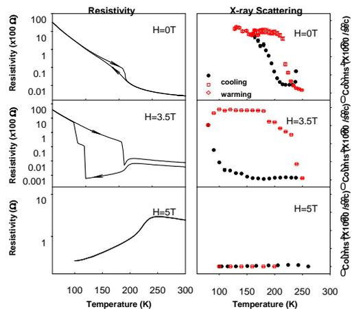
Figure 1 the temperature dependence of charge ordering under external magnetic field of  $H=0, 3.5$  and  $5$  Tesla. Also shown is the resistivity of the same sample in the corresponding magnetic fields.
