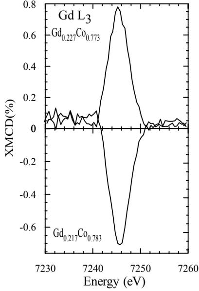
Fig.1: XMCD signal at the Gd  $L_3$ -edge in  $Gd_{0.227}Co_{0.773}$  and  $Gd_{0.217}Co_{0.783}$  alloys at 300 K.
