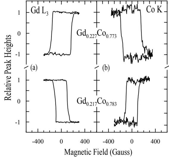
Fig.3: Element specific magnetic hysteresis at a) Gd  $L_3$ -edge b)Co K-edge in  $Gd_{0.227}Co_{0.773}$  and  $Gd_{0.217}Co_{0.783}$  alloys at 300 K.
