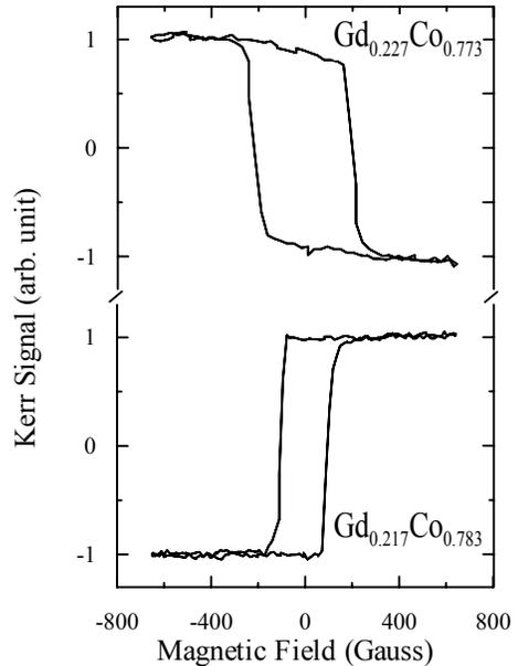
Fig.4: SMOKE measurement in  $Gd_{0.227}Co_{0.773}$  and  $Gd_{0.217}Co_{0.783}$ alloys at 300 K.
