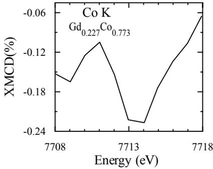
Fig.2: XMCD signal at the Co K-edge in  $Gd_{0.227}Co_{0.773}$  alloy at 300 K.
