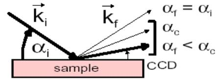
FIG. 1. Sketch (side view) of the geometry used in the experiment. The out-of-plane directions, which are referred to as the x-coordinate or  $\phi$ -angle, lie perpendicular to the drawing plane and are not shown here.
