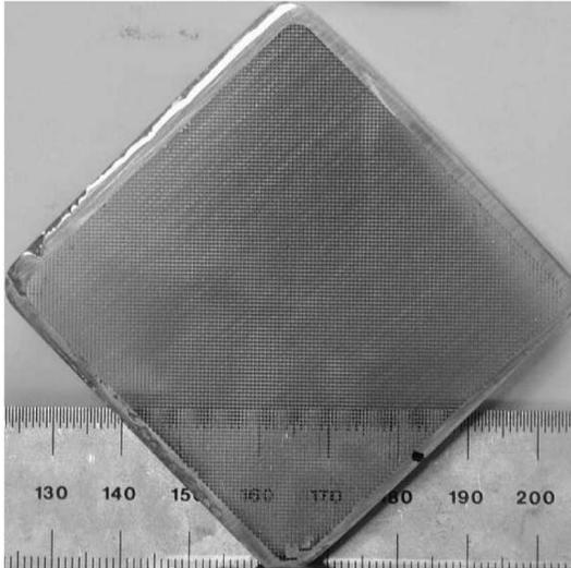
FIG. 2. Photo of a focused copper grid.
