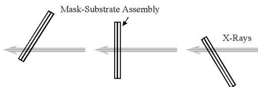
FIG. 1. The position of the mask-substrate assembly at different orientations during the x-ray exposure.
