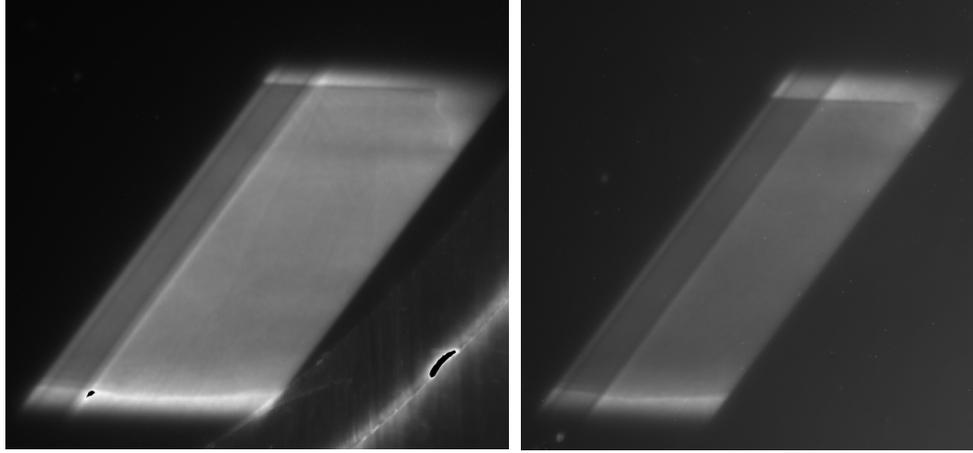
FIG. 1. X-ray images of Fe sample before and after the transition from bcc (left) to hcp (right) phase.
