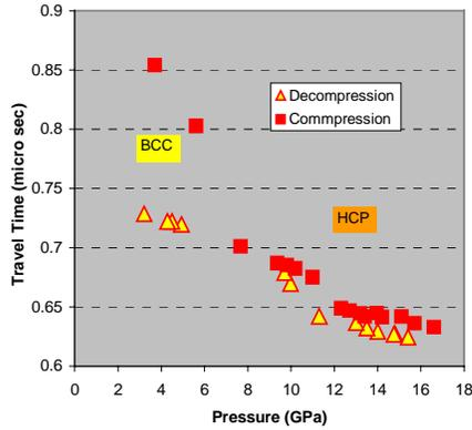
FIG. 2. S wave travel time as a function of pressure.
