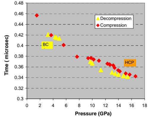
FIG. 3. P wave travel time as a function of pressure.
