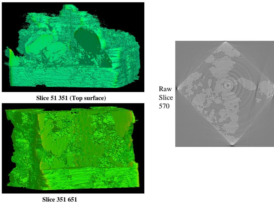
FIG. 2. XCT of vacuum-plasma-sprayed titanium coating. Scale is approximately  $600 \mu\text{m}^2$  on a side.
