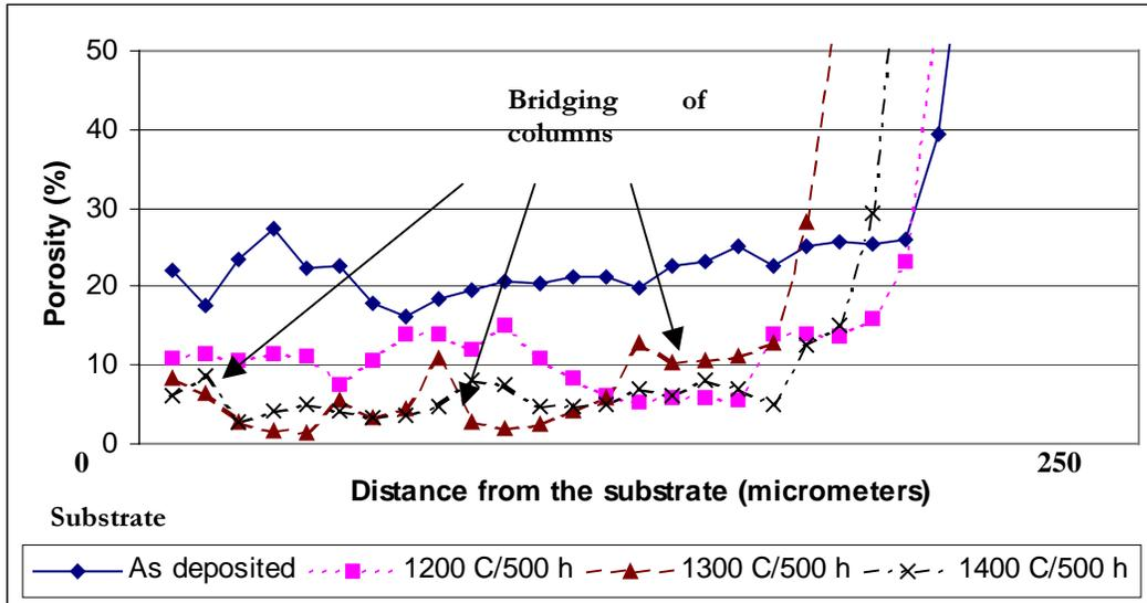
FIG. 1. Influence of exposure temperature on porosity variation along the thickness of the coatings.
