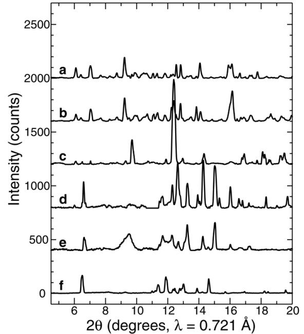
FIG. 3. Radially integrated and background-subtracted  $\mu$ XRD patterns from areas of high U concentration in samples 61A (a-c) and 67A (d-f).
