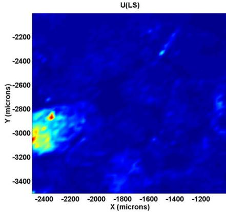
FIG. 1. Example  $\mu$ SXRF map of the uranium distribution in sample 61A. The U  $L_a$  fluorescence was measured with a log spiral bent Laue analyzer. Red corresponds to the highest U concentration.
