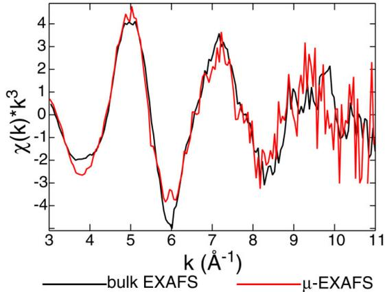
FIG. 2. Comparison of  $\mu$ EXAFS spectrum of a  $20 \times 20 \mu\text{m}$  area of high U concentration in sample 61A to the bulk EXAFS spectrum from the same sample [2].
