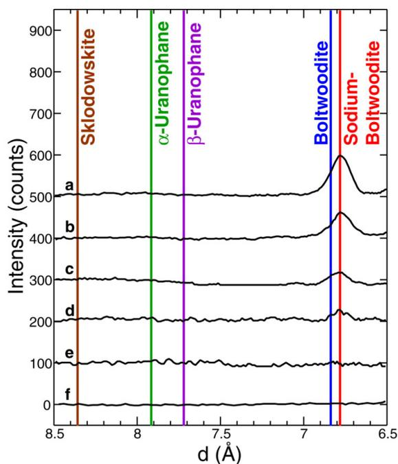
FIG. 4.  $\mu$ XRD patterns from areas of high U concentration in samples 61A (a-c) and 67A (d-f) plotted versus  $d$ -spacing for the region of the most intense lines of uranophane group minerals.
