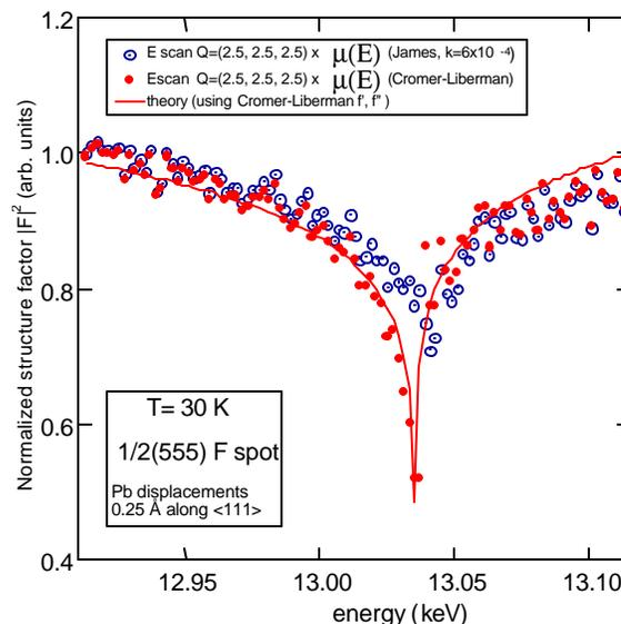
FIG. 3. Results after correction for absorption data and fitted energy dependence of the structure factor.
