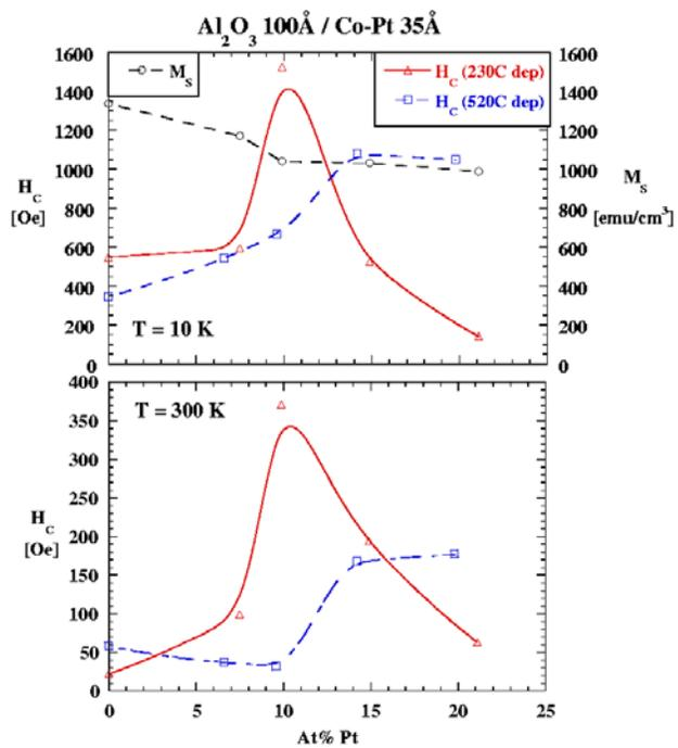
FIG. 1. Saturation magnetization ( $M_S$ ) and coercive field ( $H_C$ ) vs. composition for  $Co_{1-x}Pt_x$  ( $x = 0.0-0.2$ ) discontinuous films.
