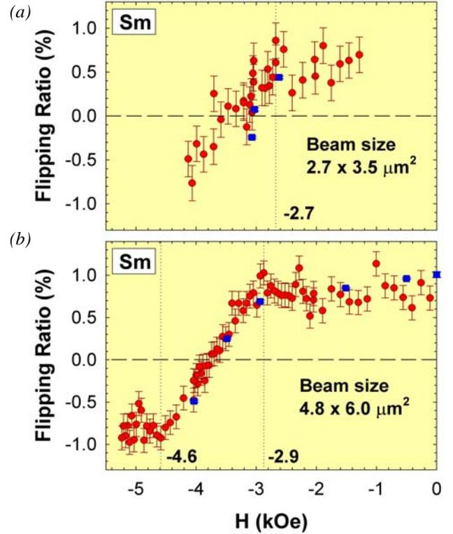
FIG. 2. Local remanent hysteresis (circles) measured by XMCD for the beam-size areas of (a)  $2.7 \times 3.5 \mu\text{m}^2$  and (b)  $4.8 \times 6.0 \mu\text{m}^2$  of the SmCo layer. Averaged remanent hysteresis (squares) calculated from the magnetization for the entire area in Fig. 1.
