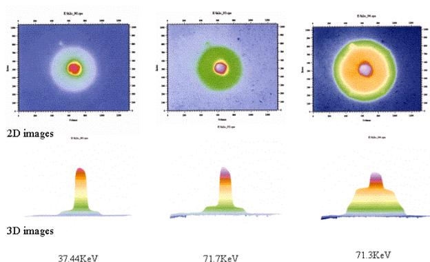
FIG. 1. X-ray radiograph of a water sample in a Re gasket with different x-ray energies.
