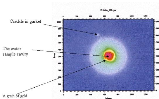
FIG. 2. 2-D x-ray radiograph of a water sample.
