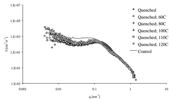
FIG. 1. Scattering plot for all UHMWPE samples.
