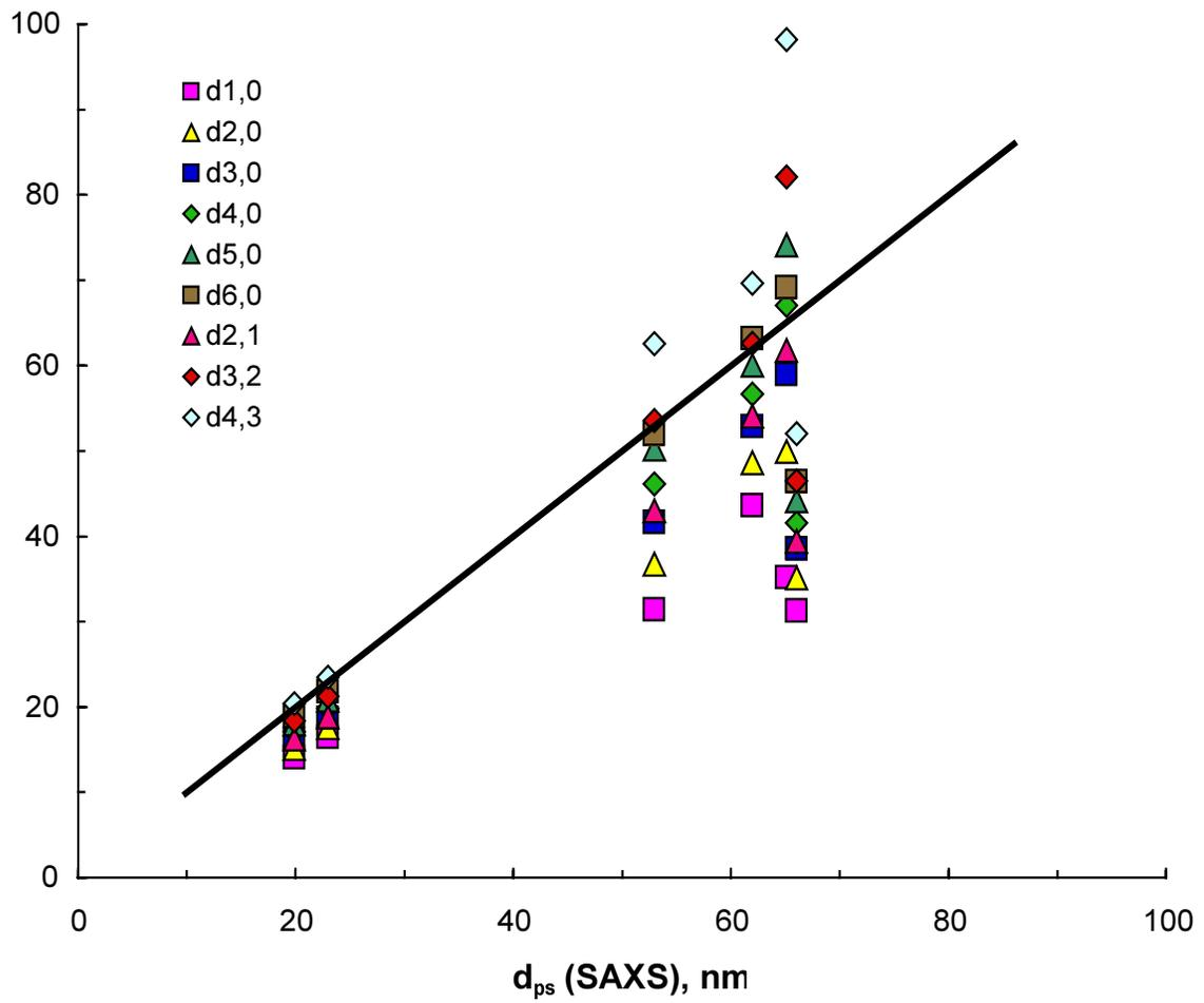
FIG. 2. Various moments of  $d_p$  for the primary particles from TEM analysis compared with  $d_p$  from USAXS data by using  $R_g$  from unified fits.
