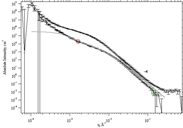
FIG. 1. Typical USAXS data for two pyrolytic silicas of different mass fractal dimension, low- $q$  power-law decay, primary particle size, prominent knee in the data, and specific surface area, power-law  $-4$  at high- $q$ . Light curve is unified fit from using a UNI-CAT-developed user software package. (Fit range is shown by circle and square superimposed on data.)
