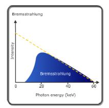
The maximum energy will correspond to the maximum high voltage applied to the X-ray tube. The maximum X-ray intensity occurs at about one-third of the maximum energy. For example, a 60 kV tube voltage will generate mostly 20 keV X-rays.
