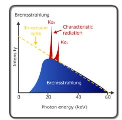
Although the X-rays have not yet passed through a filter, the very low energy X-rays are missing. This is because the X-ray tube window acts as a filter.
