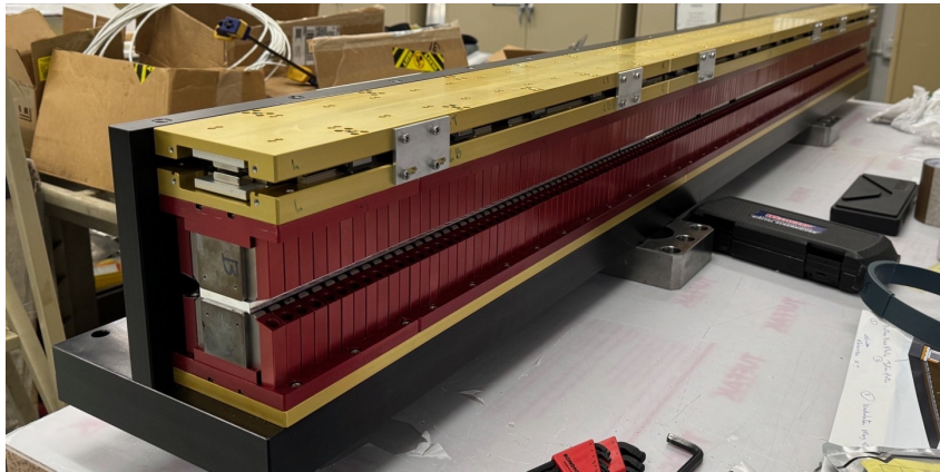
Planar FNAPU prototype undergoing magnetic testing
