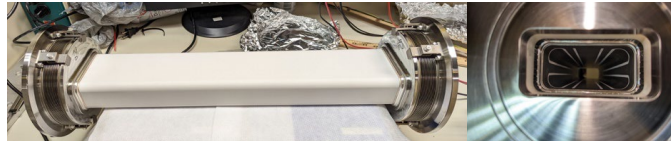
PAR kicker chamber with innovative Ti coating
