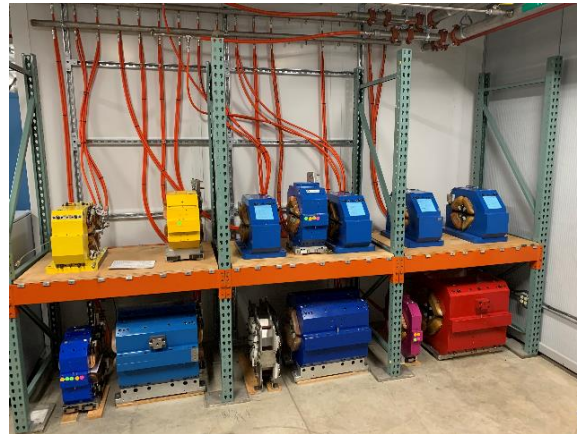
Power Supply Controller Test Stand (top) and Power Supply Magnet Loads (bottom)
