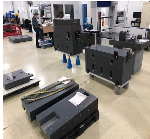
Canted GRID XBPM support system under fabrication at Tru-stone, MN
