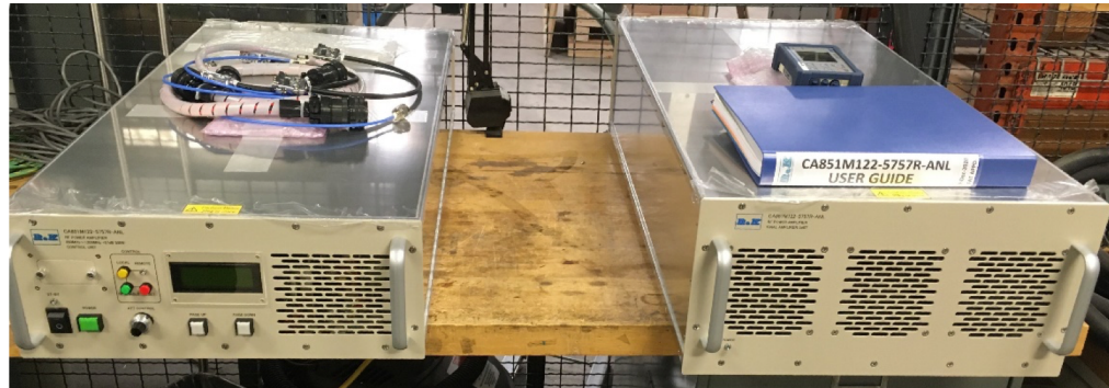
Control unit (left) and power unit (right) of first article longitudinal feedback power amplifier.
