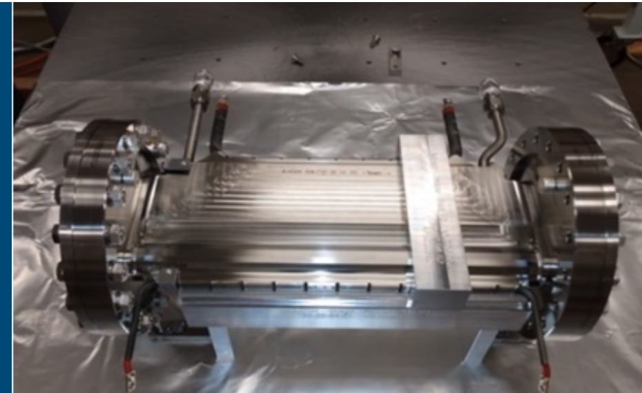
First article keyhole vacuum chamber upon delivery to Argonne
