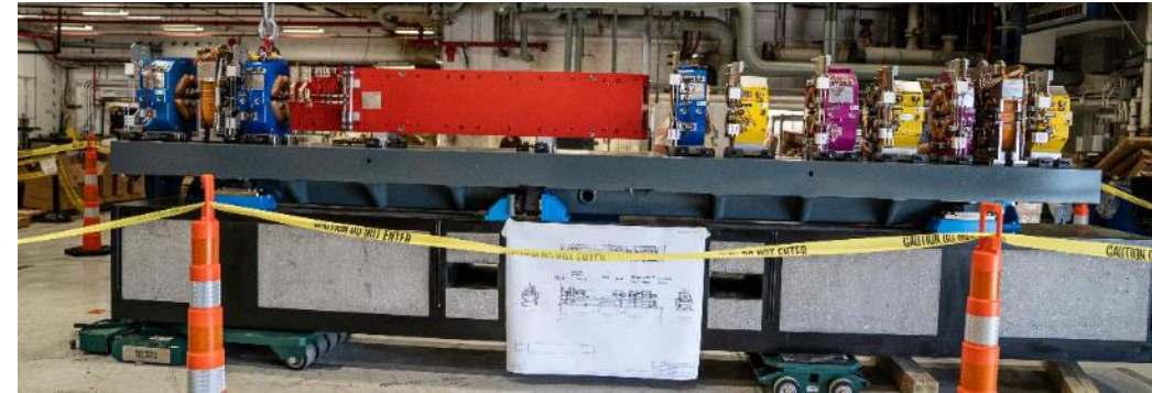
1 st DLMA girder assembly with measured flatness of 10 microns (30 microns rms alignment tolerance specified).
