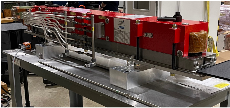
Lambertson Septum at ANL on measurement stand.
