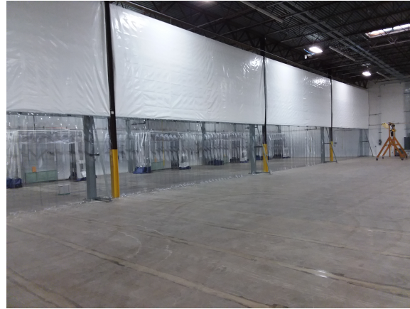
Retractable clean rooms & cranes inside module assembly area (Bay 1 of 3)
