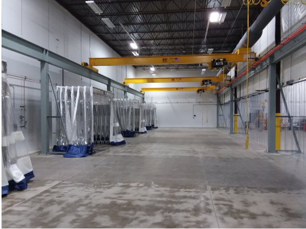
Retractable clean rooms & cranes inside module assembly area (Bay 1 of 3)
