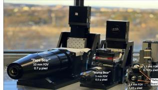
Centimeter scale FOVs are needed for whole-organism phenotyping of small model systems and tissue specimens from larger organisms including humans. This required custom large-FOV optics based on photolithography lenses and 150 MP chips. (See Yakovlev et al. poster)
