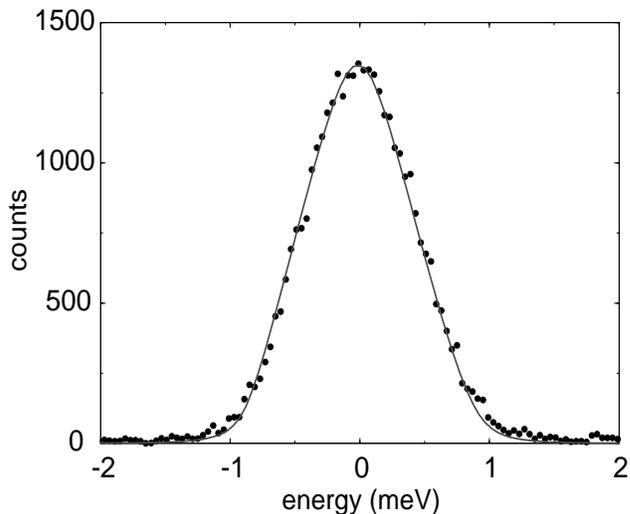
FIG. 2. Energy resolution function of the monochromator as measured by nuclear resonant scattering from  $^{151}\text{Eu}$ . The energy width is 1.0 meV FWHM.
