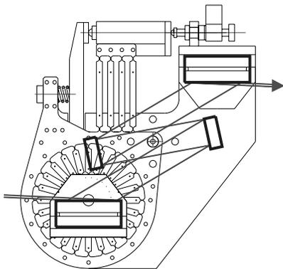
FIG. 1. Design of the high-resolution monochromator using silicon  $+(4\ 4\ 0)$ ,  $+(15\ 11\ 3)$ ,  $-(15\ 11\ 3)$ ,  $-(4\ 4\ 0)$  crystal reflections.
