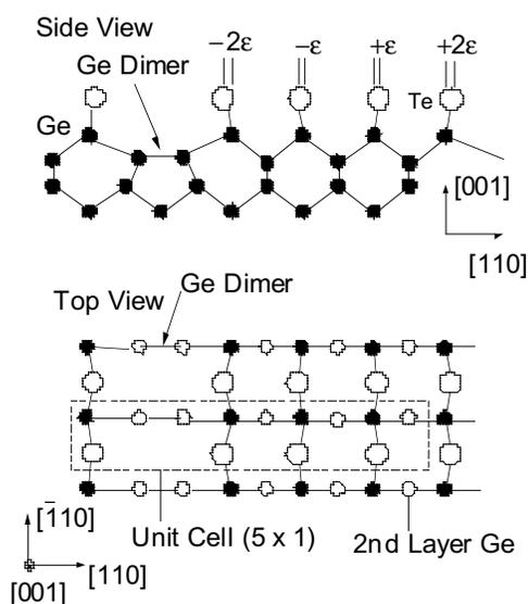
Figure 1: Te missing-row model for the Ge(001):Te 1 x 1 surface.
