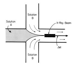
Figure 1: A cross sectional schematic of the rapid fluid mixer.
