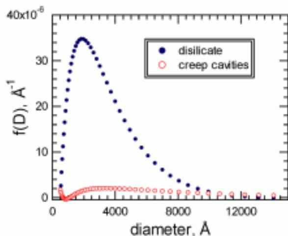
Figure 1: Size distributions of Yb disilicate and voids in a sample tested for 50 hours. While the size distributions are similar, the volume fraction of disilicate particles is much greater than the volume fraction of the voids.
