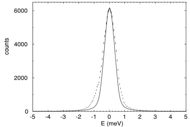
Figure 3: The measured energy response function (vertical bars,  $\text{FWHM} = 0.98 \text{ meV}$ ) of the monochromator  $\text{Si}(444) - (121212)$  compared with a simulation (solid line, with  $\text{FWHM}$  of  $0.80 \text{ meV}$ ).
