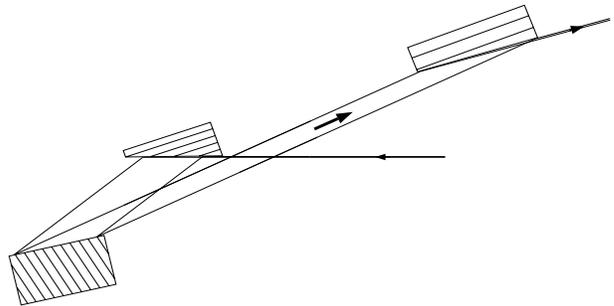
Figure 4: The  $1 \text{ meV}$  monochromator in a 3-crystal setup.
