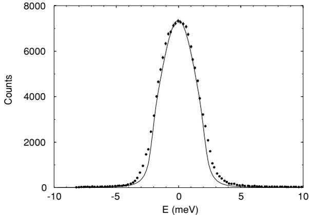
Figure 2: The measured energy response function (dots,  $\text{FWHM} = 3.6 \text{ meV}$ ) of the  $\text{Si}(400) - (121212)$  monochromator, compared with a simulation (solid line, the vertical scale is arbitrary).
