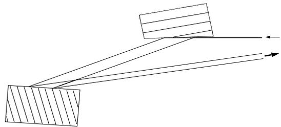
Figure 1: The monochromator Si(400) – (121212).
