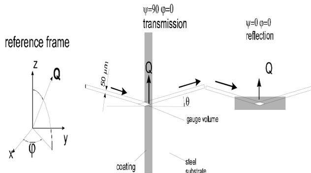
Figure 1: Schematic of beam dimensions and sample orientations.
