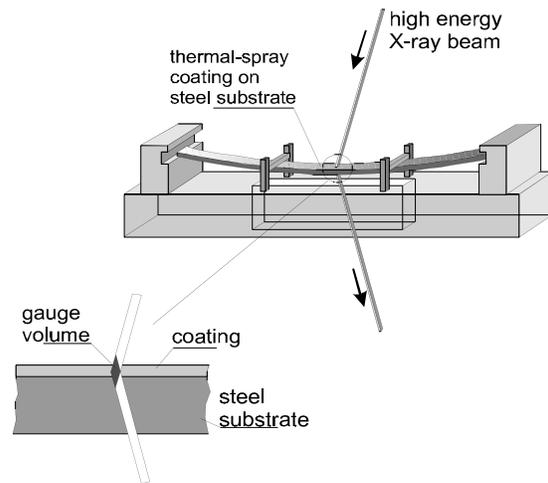
Figure 2: Experimental setup of the bending experiments. The actual scattering plane was horizontal.
