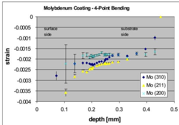
Figure 4: Molybdenum coating in a four-point bending experiment. The measurement was conducted in transmission geometry.
