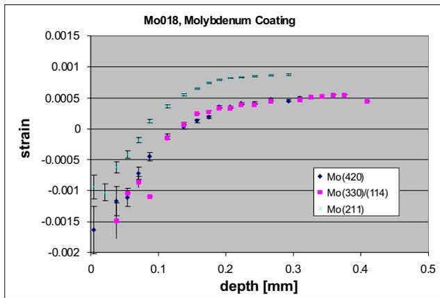
Figure 3: In-plane strain measured in transmission on a Mo coating.
