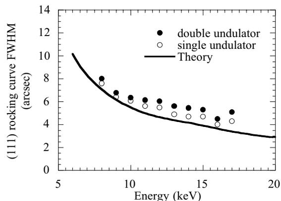
Figure 1: FWHM of the (111) double-crystal rocking curve as a function of energy for one and two undulators at 11 mm gap.
