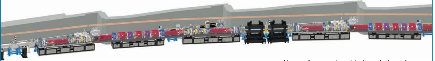
Above: A computer-aided rendering of a typical APS-U storage ring sector showing the MBA-lattice configuration of red, blue, and purple electromagnets and associated components. Rendering by the AES Design and Drafting Group.
