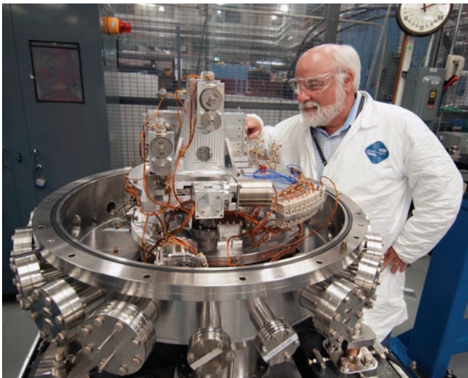
Above: Technicians from the APS Accelerator Systems Division Magnetic Devices Group and the APS Engineering Support Division Survey and Alignment Group working on a helical superconducting undulator insertion device. Super-conducting undulators are now in operation in the APS storage ring and are a key component of the APS-U. They produce stronger magnetic fields and thus higher-energy x-rays than conventional permanent magnetic undulators having the same period lengths.
