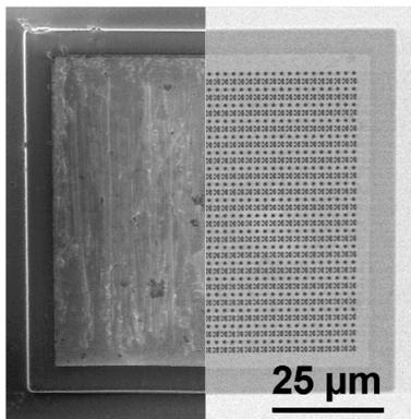
The figure above shows two views of the same area of interest in a 10-micrometer-thick semiconductor bond pad. At left is a conventional SEM image. At right is an SCEM image of the same area, showing details of the internal microstructure that are hidden from view in the SEM image.
