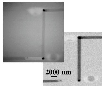
This figure compares images obtained from the same area of an electromigration void at an interconnect using SCEM (left) and STXM (right). This result illustrates that the resolution of the SCEM rivals that of the STXM in a device that can be procured and operated at a fraction of the cost.
