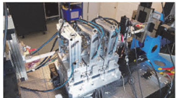
R&D collaborative project with French industry: magnetic bench (pulsed wire) for the measurements of an original concept of hybrid permanent magnet based quadrupole.
