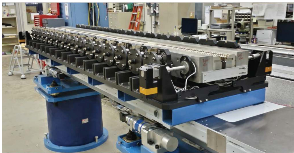
Figure 5.57. The 3 m prototype of HGVPU built for LCLS II at APS.
