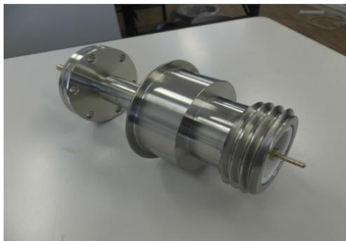
Figure 4.166. Finished prototype feedthrough.
