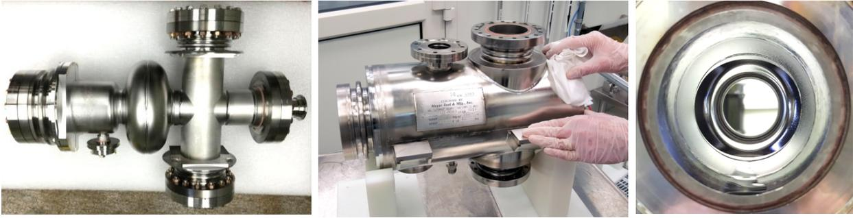
Figure 4.211. 1.4 GHz higher-harmonic cavity. Left: bare cavity weldment. Center: Cavity encapsulated within helium vessel. Right: View along cavity bore.
