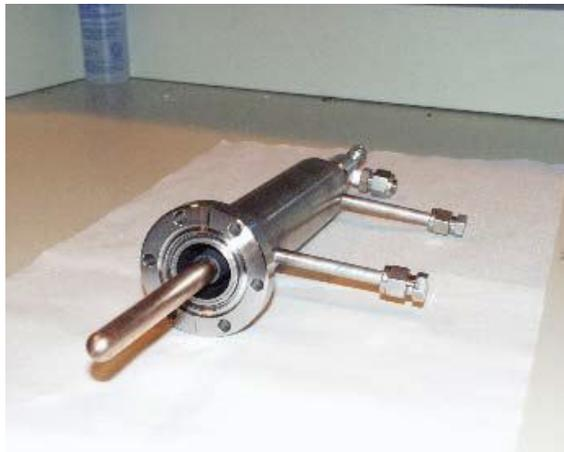
*Figure 4.210. The APS HOM damper. Four of these dampers are installed in the Sec. 36 cavities.*
