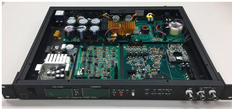
Figure 4.150. Prototype fast corrector power supply.
