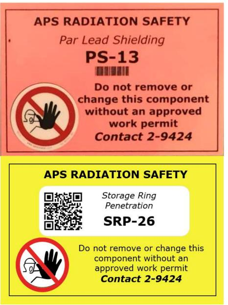
The contact 2-9424 on this example is the telephone extension for the Main Control Room. The QR code in the tag label leads to the CDB entry for the component.
