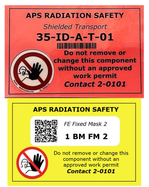
The contact 2-0101 on this example is the telephone extension for the on-duty Floor Coordinator. The QR code in the yellow tag label leads to the CDB entry for the component.
