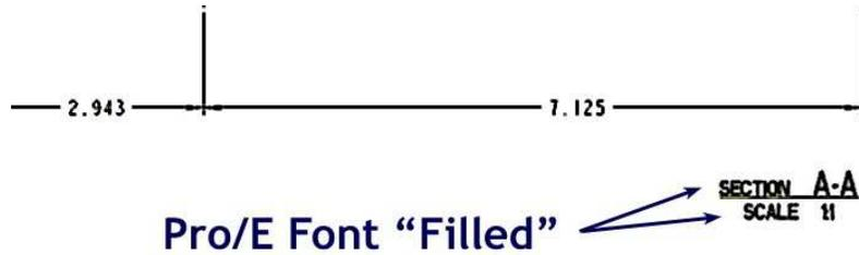
**Figure 1-1:** Pro/E defaults to proper font sizes for view identifier text, but designers must change font type.
