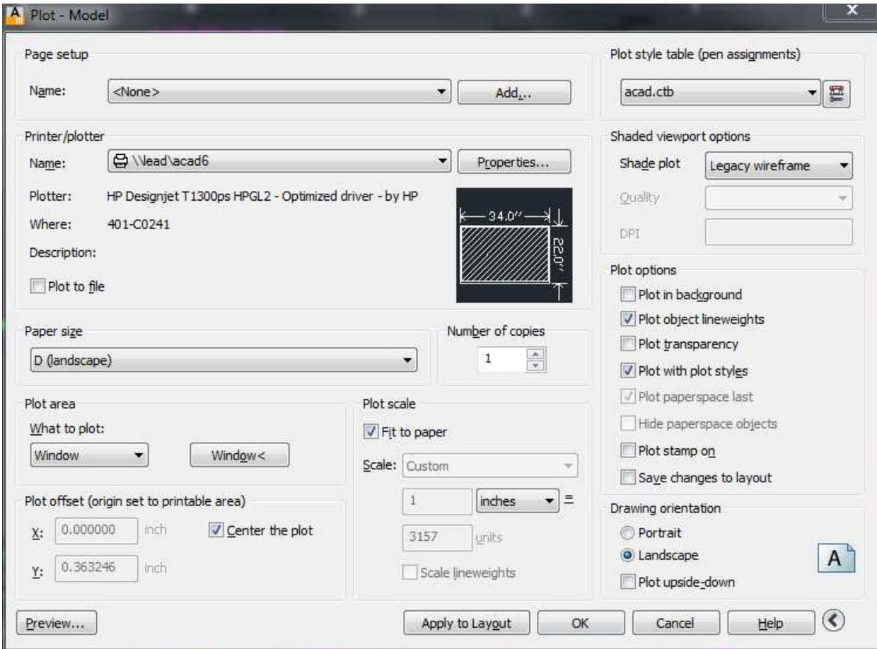
Figure 11–2: AutoCAD plot dialog.
