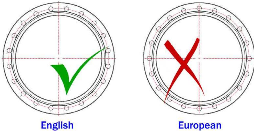
**Figure 8-1:** Proper orientation for aligning flanges (to be followed unless spatial interference conditions exist).
