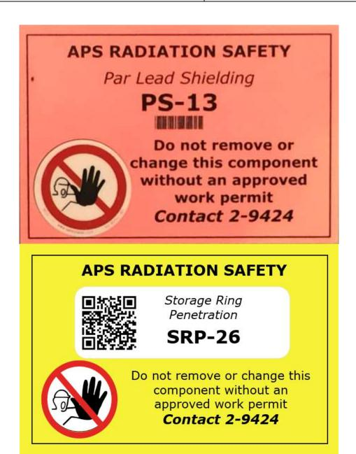
The contact 2-9424 on this example is the telephone extension for the Main Control Room. The QR code in the tag label leads to the CDB entry for the component.
