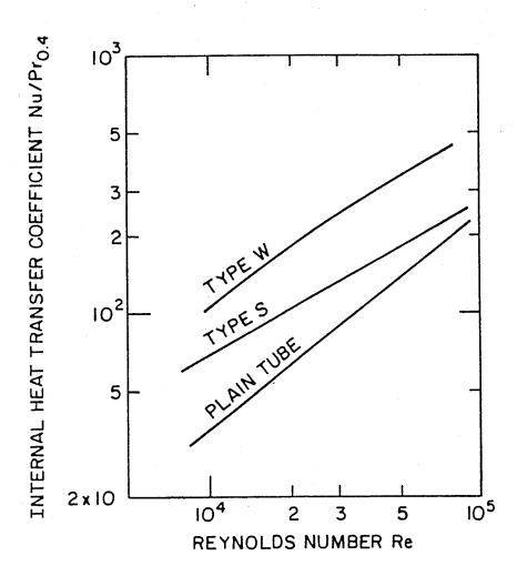
Fig. 4. Internal heat transfer coefficient of Hitachi Thermofin-SP tube [6].
