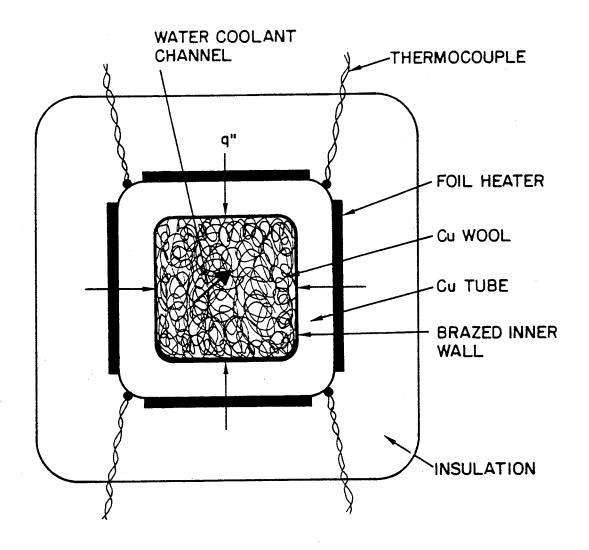
Fig. 5. Copper wool filled rectangular heavy-wall copper tubing.
