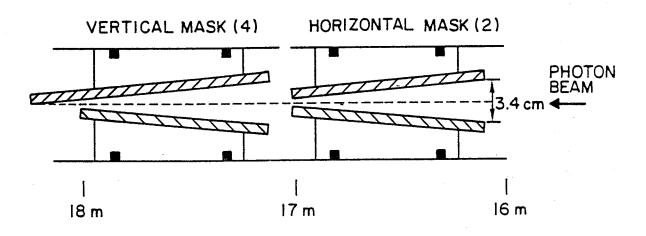
Fig. 2. Partial layout of a fixed vertical and fixed horizontal mask assembly.
