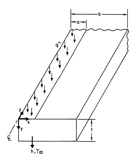
Fig. A.1. Half absorber plate geometry of the problem formulation.
