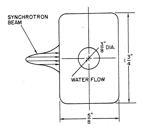
Fig. 3. FMA copper tubing for the NSLS X-17 wiggler.
