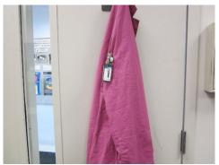
Incorrect! The dosimeter was left on a lab coat, which is near a radiological work area. It may record high background radiation exposure while not being worn.
