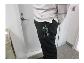
Incorrect! This dosimeter is too low. Do not hang it off a key chain or clip. Remember, it should be centered between the neck and waist and facing away from you.
