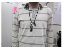
Incorrect! The dosimeter is facing backwards. The measured skin dose from low penetration radiation will be inaccurate.
