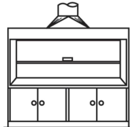
b) *For hoods equipped with horizontal sashes, slide the sashes to minimize the openings, keeping a panel between you and your work.*
