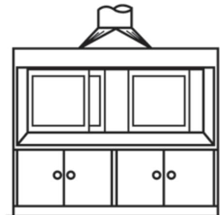
5. **Keep chemical hood sashes closed to a six inch opening when the hood is not in use.** *The sash will act as a shield in the event of an unexpected release, but the opening will maintain a point of air exhaust for the lab.*
