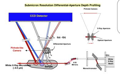
Differential-Aperture X-Ray Microscopy (DAXM) Measurement of Local Crystal Structure With Submicron Resolution In Three-Dimensions
