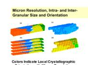
Orientation with Micron Resolution Grain-Orientation and Morphology in Polycrystalline Al
