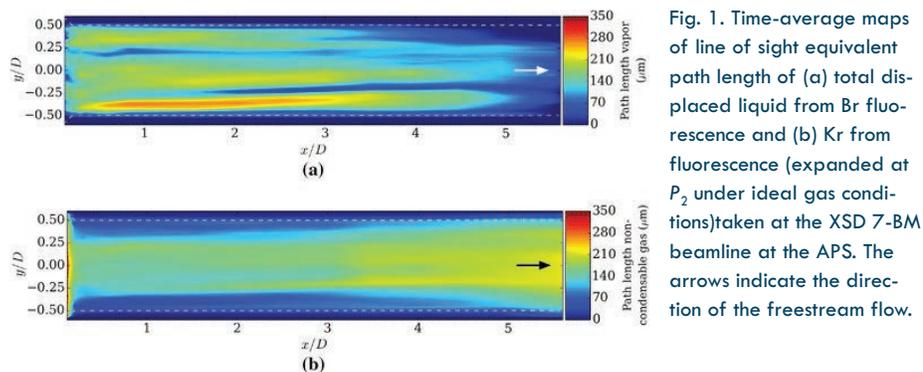
Fig. 1. Time-average maps of line of sight equivalent path length of (a) total displaced liquid from Br fluorescence and (b) Kr from fluorescence (expanded at  $P_2$  under ideal gas conditions) taken at the XSD 7-BM beamline at the APS. The arrows indicate the direction of the freestream flow.
