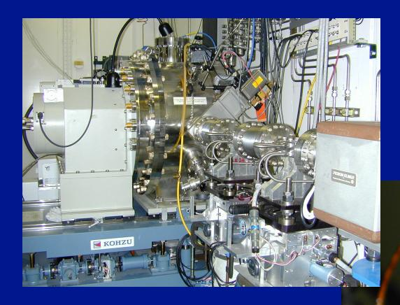
Kohzu high-heat-load monochromator consists of two water-cooled Diamonds
