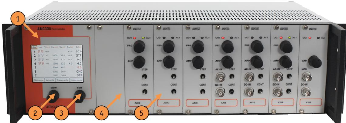
**Figure 1:** Front panel of the ANC300 with seven ANM modules in place.
