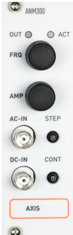
The ANM300 module is an open loop positioning and scanning module. The nominal output voltage is unipolar from 0 to 150 V. The outputs are protected against short-circuits and have a current limiter in order to protect them. The following functions are available (see schematic graph below):
