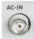
When switching on the AC-IN feature, a voltage of up to 10 VAC can be added to the output (gain 1, no amplification) using the AC-IN BNC on the frontplate of the module. Additional filtering can be switched on, with a second order low pass filter with approx. 16 Hz, 160 Hz, or no filter.
