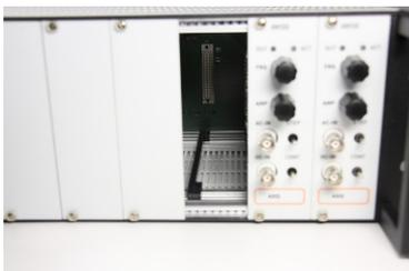
After mains and all other cabling have been removed, open the cover of a free slot in the ANC300. Carefully insert the module taking care not to touch the electronics with bare hands to avoid damages due to static electricity.
