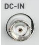
There are two BNCs on the module frontplate, labeled DC-IN and AC-IN. The DC-IN input accepts  $-10 \dots +10$  V, while the output is (nominally)  $0 \dots +150$  V. The gain is 15 (see Figure 6).
