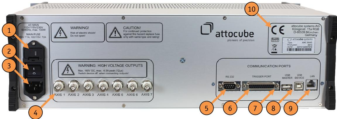
**Figure 3:** Back panel of the ANC 300 piezo positioning electronic.
