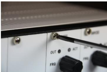
To open the housing, unscrew the two screws on the front side of the respective axis. The boards are connected to a backplate by a connector, so some force is required to pull them out. If possible, open a blank cover next to the module and hence get a better grip on the frontplate. Otherwise, use the BNC connectors (attach e.g. a T-piece) or the dials and carefully pull on them to withdraw the module.
