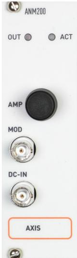
The ANM200 module is an open loop, low noise scanning module. The nominal output voltage is unipolar from 0 .. +150 V. The outputs are protected against short-circuits and have a current limiter in order to protect them. The following functions are available (see schematic graph below):
