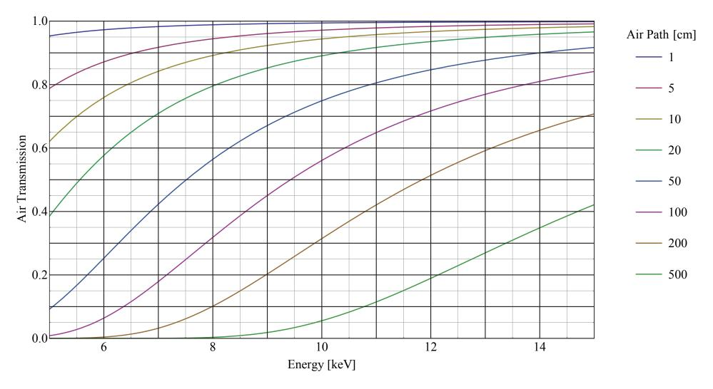
Look for the air path length in cm on the right and follow the curve to the working energy in keV on the x-axis below, read the absolute transmission on the y-axis to the left.
