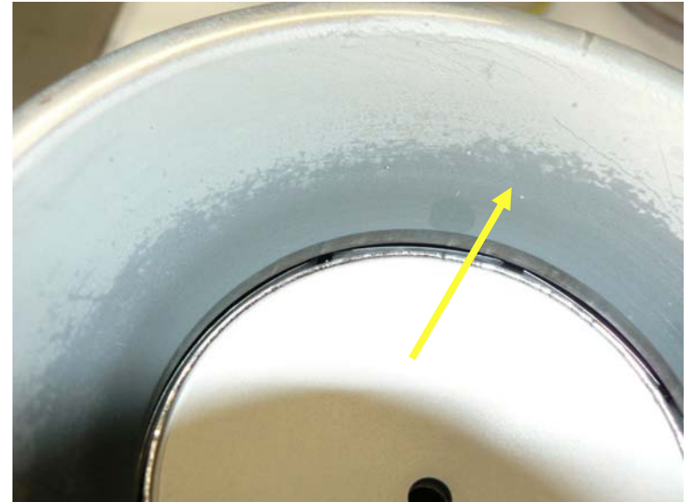
Excessive barium on cathode whenelt electrode
