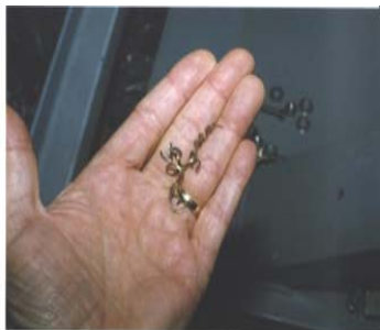
Foreign material found between collector and boiler
