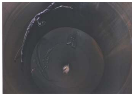
Melting on interior of collector
