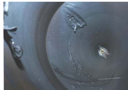
Melting on interior of collector
