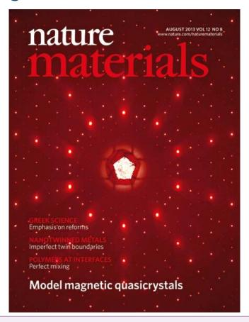
Diffraction pattern from a Gd-Cd quasicrystal showing ten-fold rotational symmetry. High-energy diffraction provides an undistorted view of reciprocal space enabling a quantitative analysis of both the Bragg peaks and diffuse scattering
