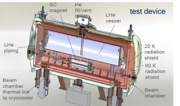
Superconducting undulator allows to increase x-ray brightness and flux in the range of 20-100 keV.
