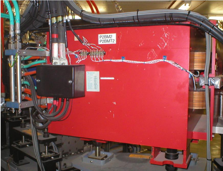
The dipoles steer the electrons around the PAR. There are 8 of these dipole magnets in the PAR. The length of the dipole is .8 m. The field strength is 1.472 T. Each dipole magnet also contains trim coils to make small magnetic corrections. The identification numbers are as follows: P1BM1, P1BMT1, P1BM2, P1BMT2, P2BM1, P2BMT1, P2BM2, P2BMT2, P3BM1, P3BMT1, P3BM2, P3BMT2, P4BM1, P4BMT1, P4BM2, and P4BMT2.
